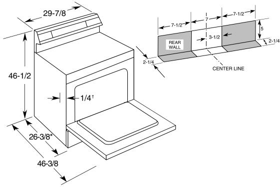
\*Dimensions from wall to front of closed oven door. Dimensions from wall to front of closed oven door handle is 28-1/2".
